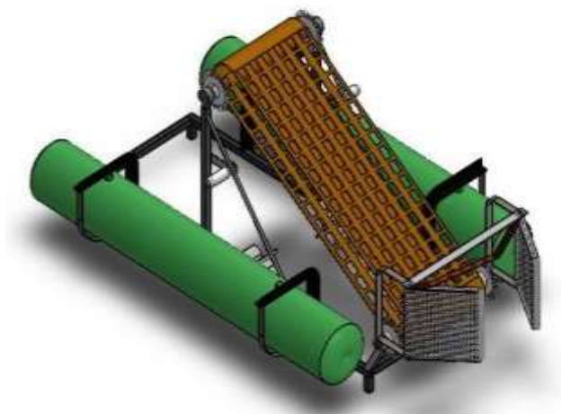
Figure 3. Assembled View of River Cleaning Machine
