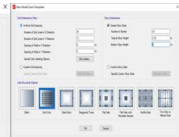
Figure 5 Floor & Dim setting
