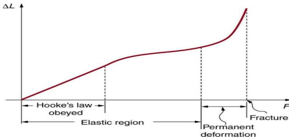
Fig. 2. Force - Deformation Curve [4]
