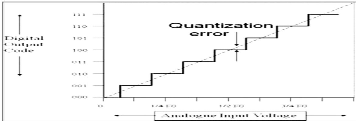
Fig.2 Variation of Quantisation error as a function of signal voltage
