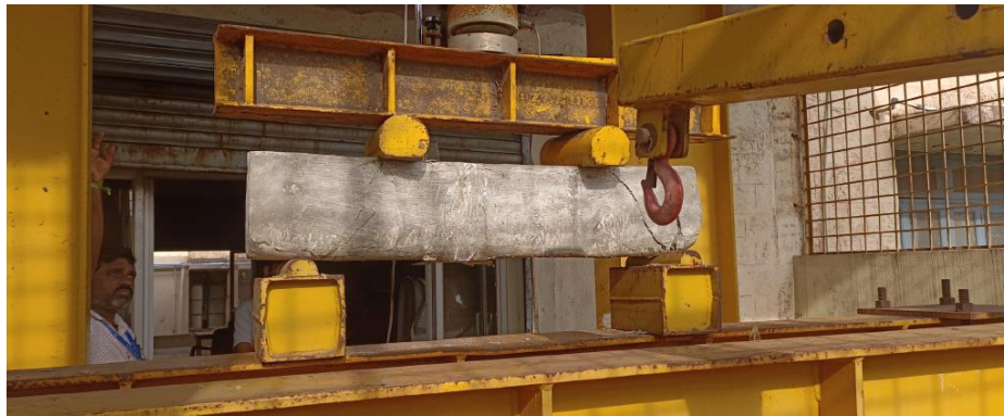
Figure 7: Testing of load framing using double point load.
