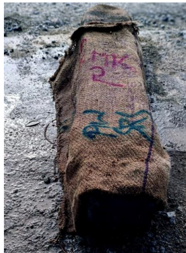
Figure 6: Curing to prepared specimen
