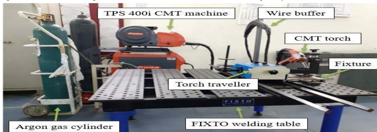
**Figure 1:** Experimental setup of CMT machine
