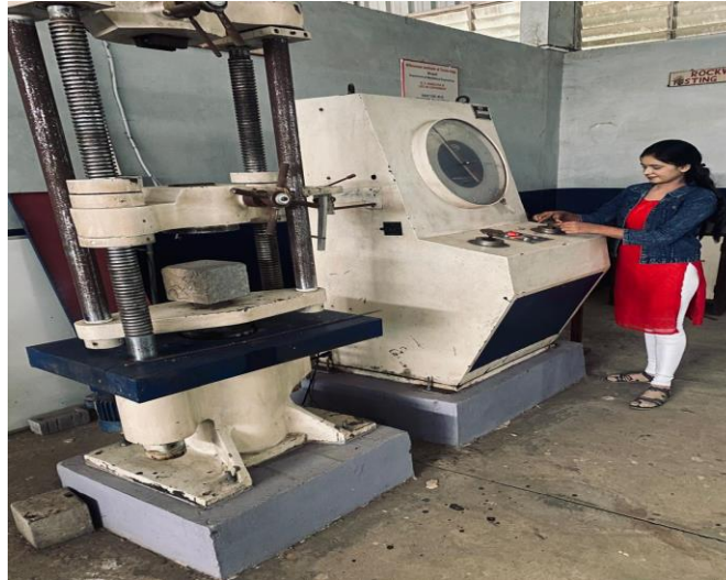
Fig. 1 Compressive Strength test
