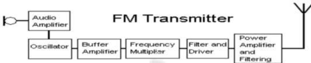
Figure 1: Block diagram of the FM Transmitter
