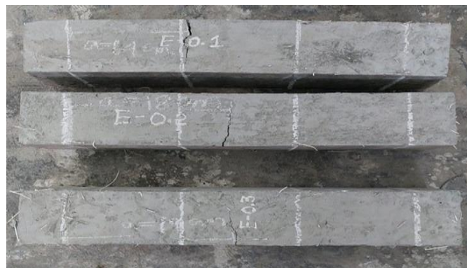
Fig 7: prisms after application of loads
