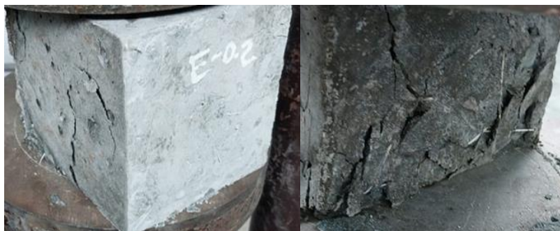
Fig 3: cubes after applications of loads
