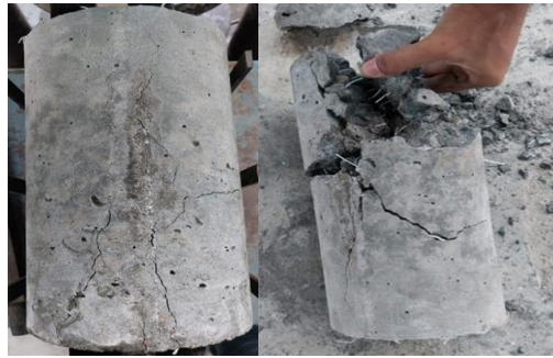
Fig5: cylinders after applications of loads
