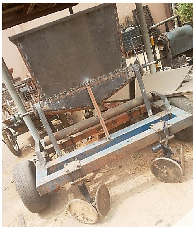
Figure 4: Fabricated solid manure injector
