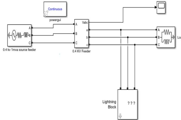
**Figure 6** Lightning impulse model
