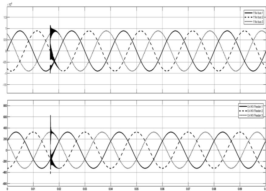
**Figure 5** Output waveform of Capacitor bank energizing model
