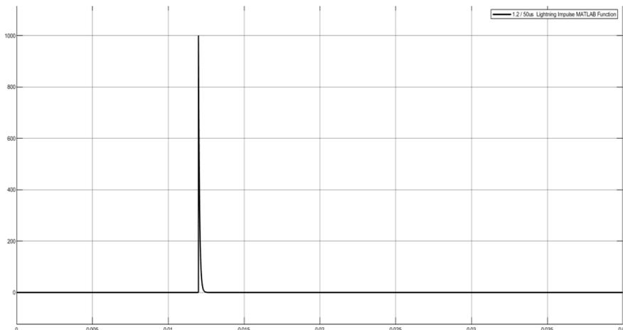
**Figure 9** Lightning impulsive waveform
