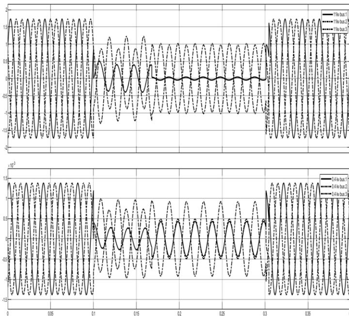
Figure 3 Voltage sag and swell caused by line-to-line fault at 11 kV line
