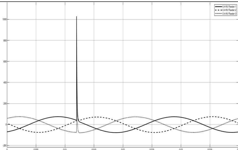
**Figure 10** Impulse transient caused by lightning near 0.4kV transmission line
