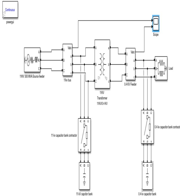
**Figure 4** Capacitor bank energizing model
