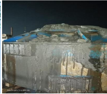
Fig RCD/BHA dismantling from Pile. Fig Slush blocked the drum outlet.
