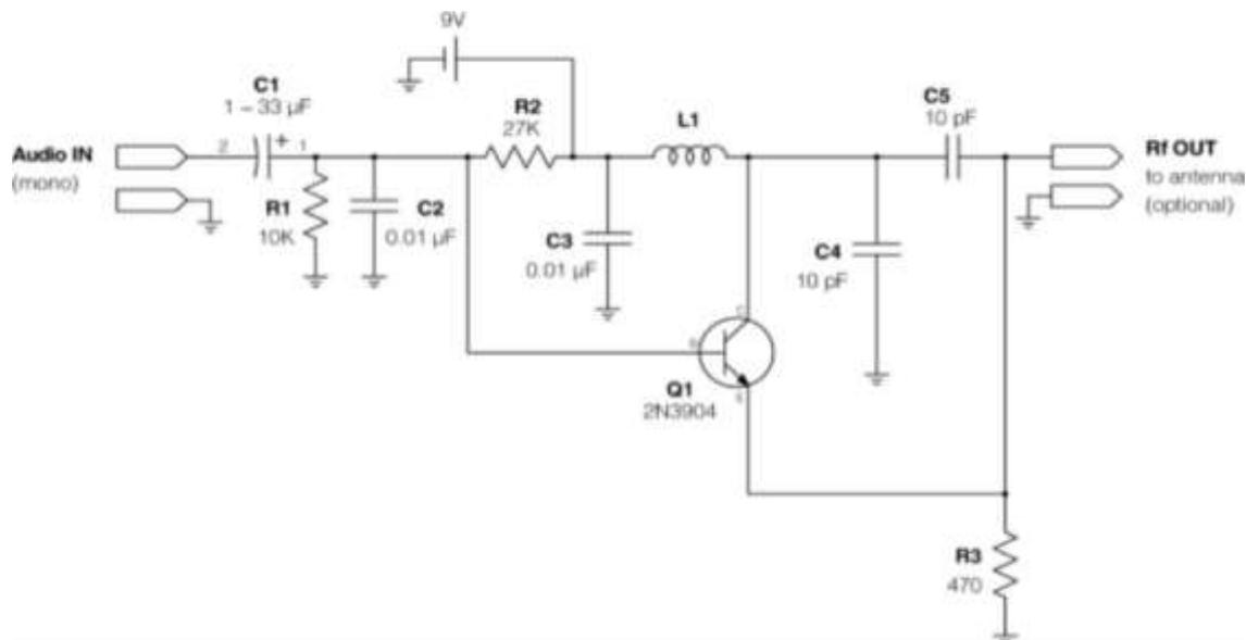
Figure 2: FM Transmitter Circuit Diagram
