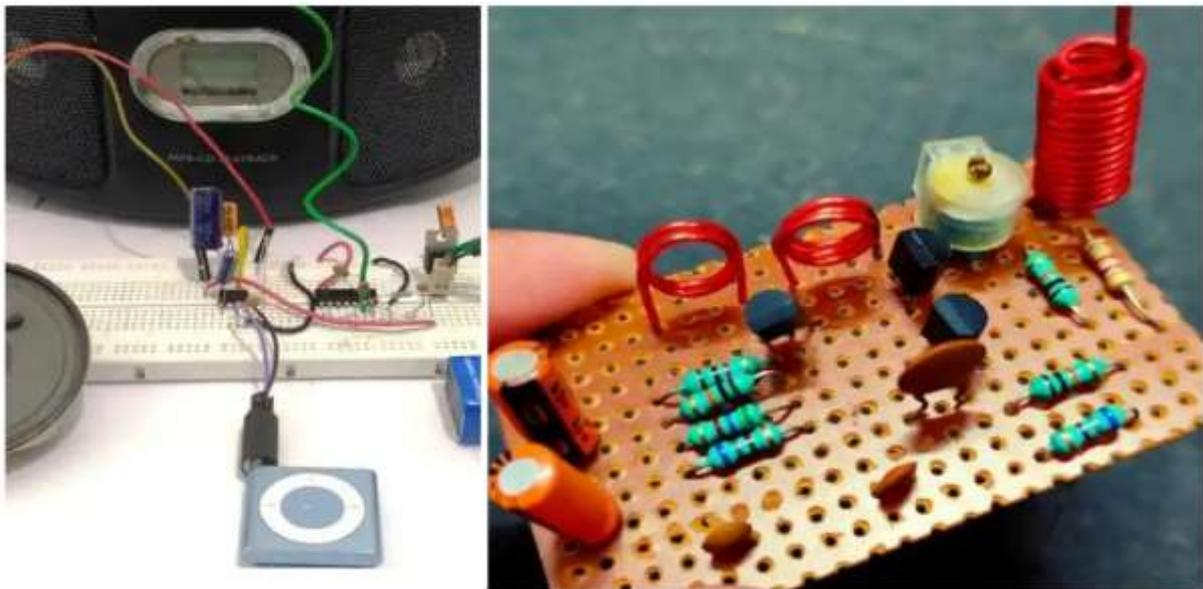
Figure 3: FM Transmitter Designed Board
