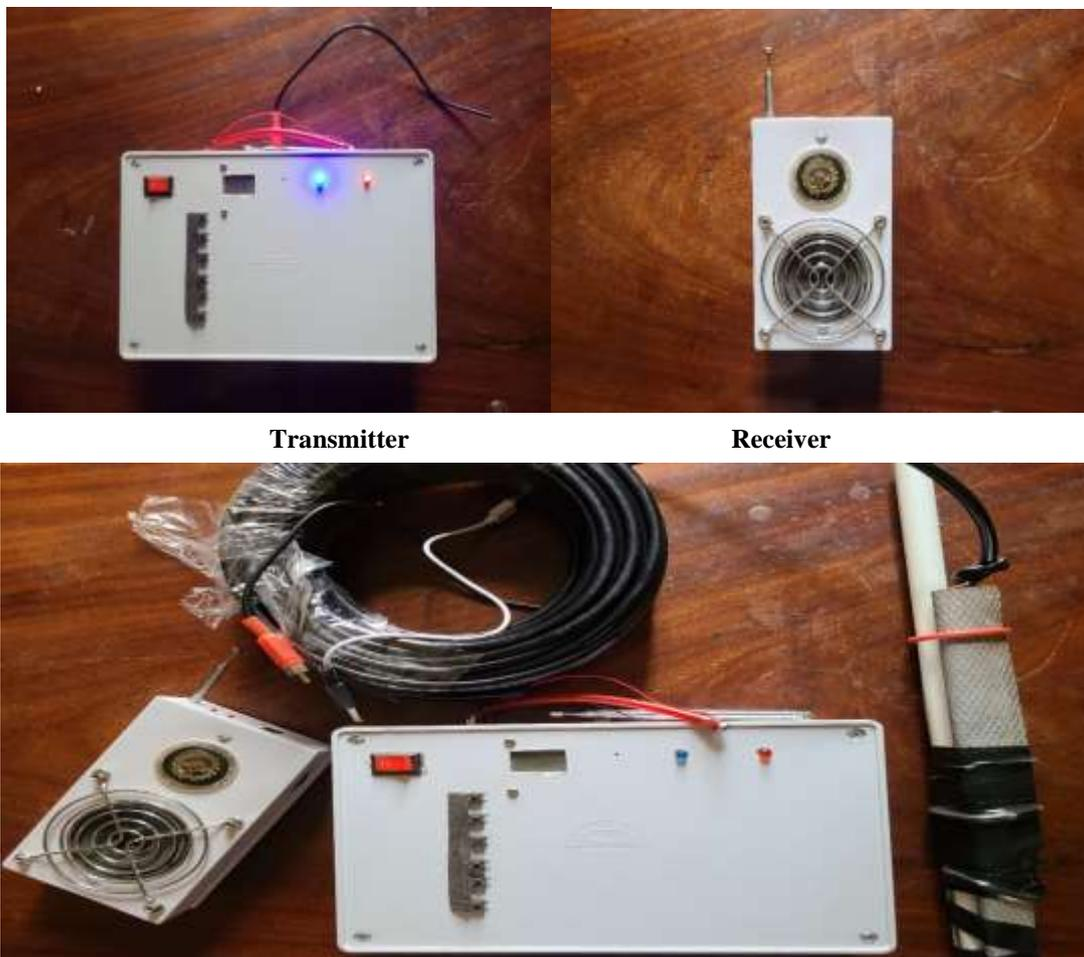
Figure 8: Designed and built FM transmitter and Receiver
